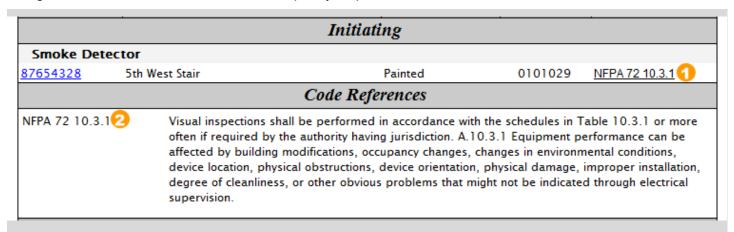
Next to each failed device will be a link that gives the chapter and section of the NFPA code (See 1 above). Click on link and the page will automatically scroll to the Code References section (See 2 above) for that device. In that section you can read the entire code text that relates to the device discrepancy. Depending on the code enforcement in your area, it will reference the 1999, 2002, or 2007 version of the codes.
